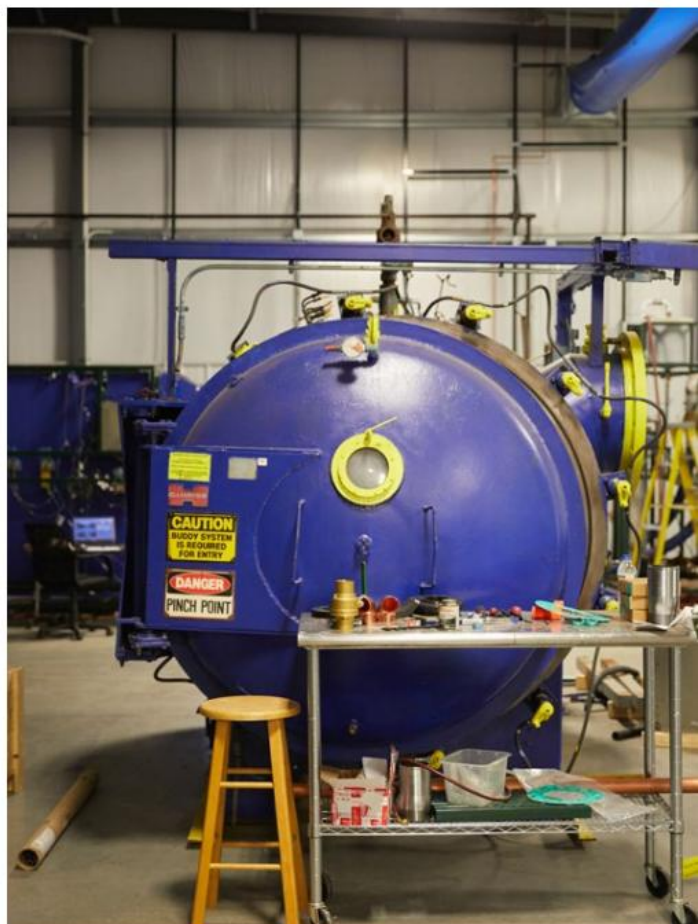
1 / Vacuum brazing furnace
