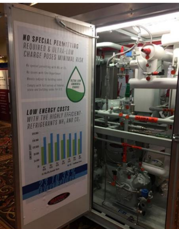
Heatcraft's low-charge ammonia rack used in NH 3 /CO 2 cascade system
