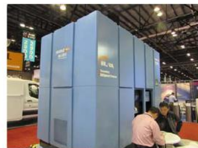
Fujian Snowman's NH 3 -CO 2 cascade system
