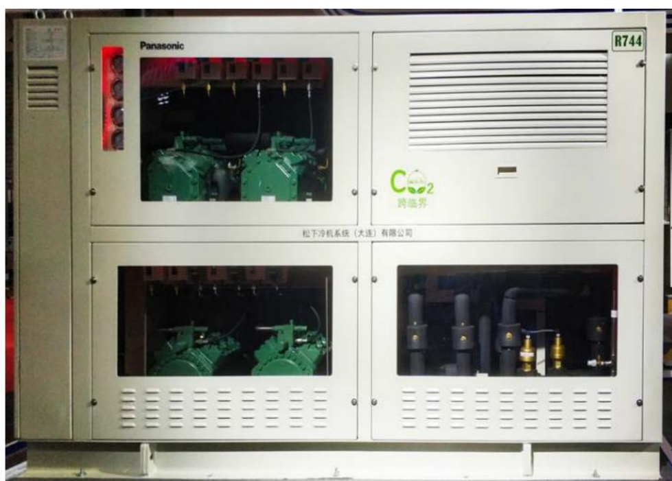
Panasonic's 80 HP transcritical CO 2 rack on display at China Refrigeration 2019
