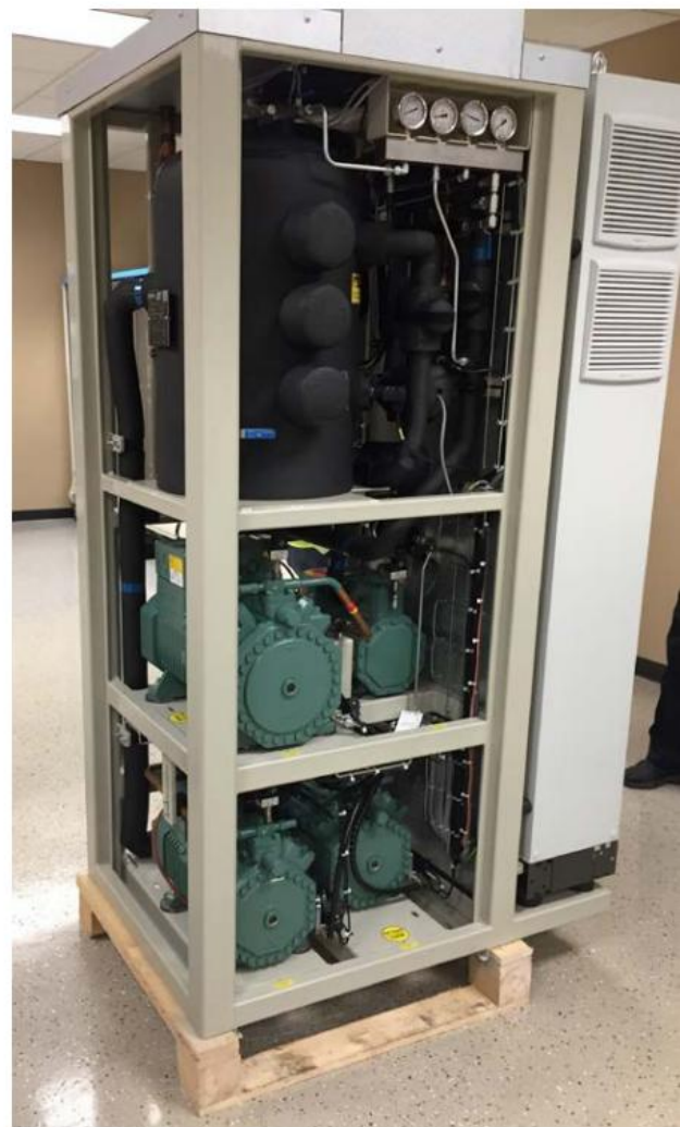
Tower distributed CO 2 system
