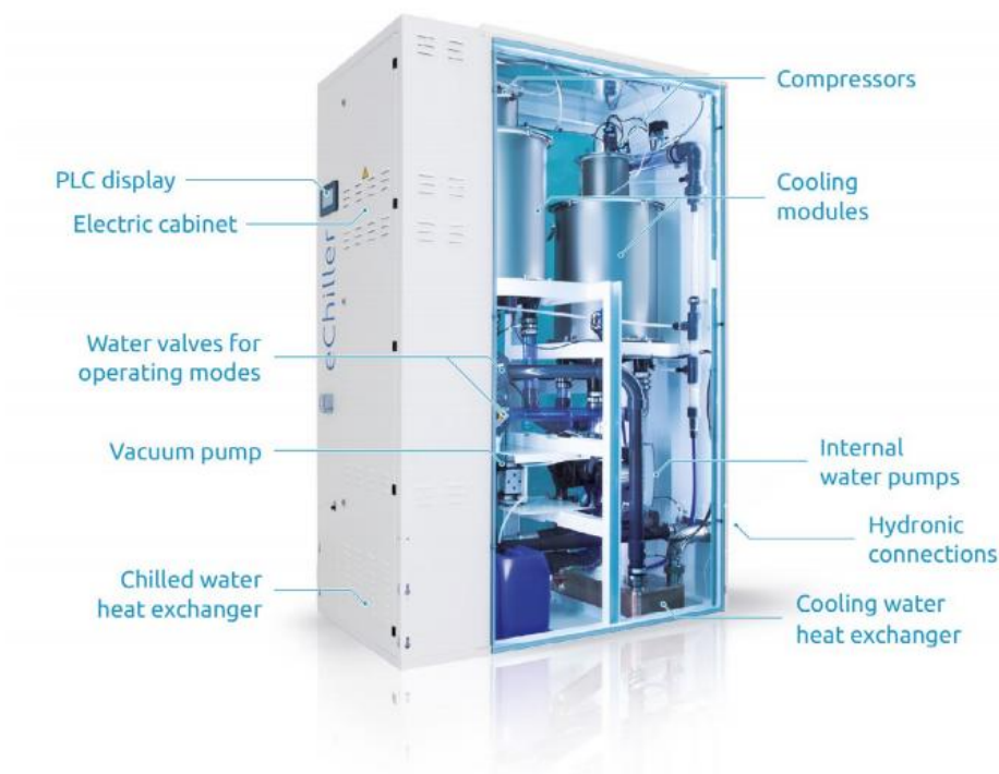
All eChiller units have the same dimensions; the capacity depends on the size and shape of the compressor impeller.
