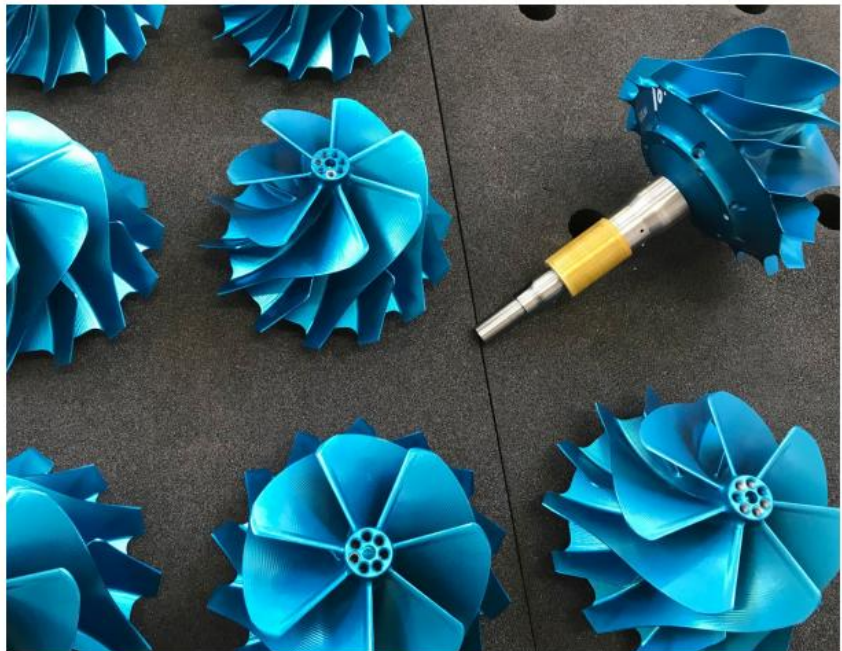
eChiller compressor impellers.
