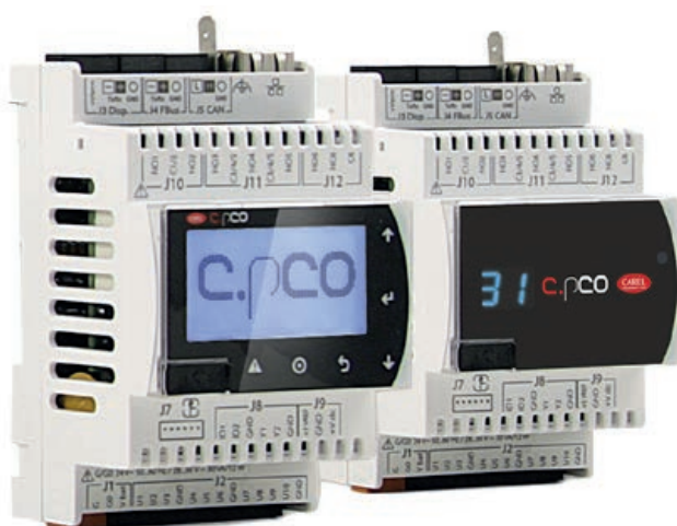
Carel's c.pCO mini controller. Photo credit: Carel.
